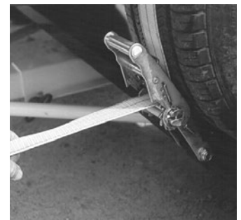
Grab excess strap and jerk hard to spin mandrel and unspool strap. ( figure c)
