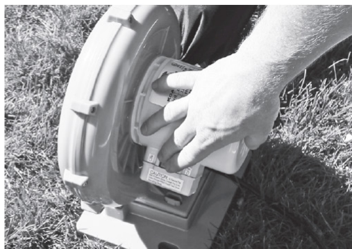
Turn on the air blower's power switch
