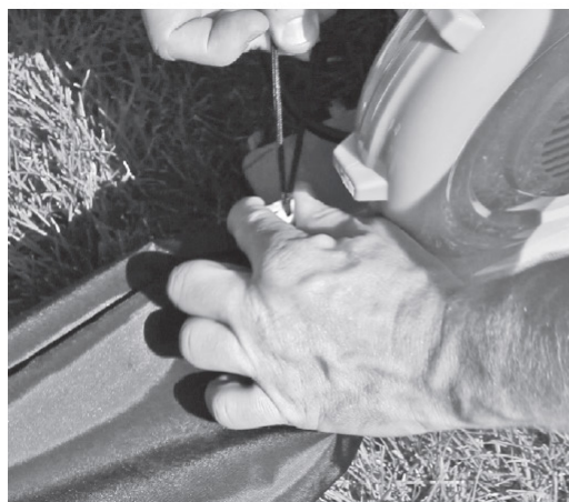
Tighten cinch cord around blower pipe
