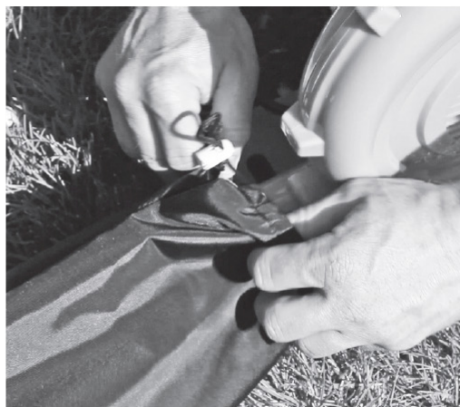
Pull intake vent over blower pipe
