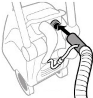
3. Turn on the switch in the accessory position. The application of cleaning solution is now controlled by the lever on the accessory tool.
