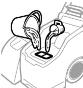
*NOTE: Periodically operate the extractor with only hot water to remove chemical residue in carpet.*
